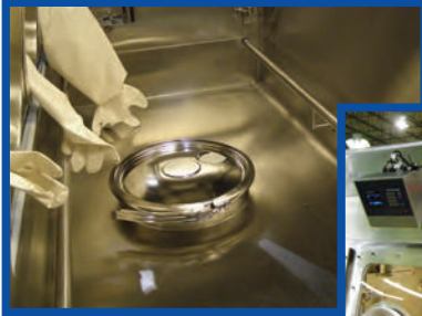
Manway Transfer Ports and Material Trolley Rail
